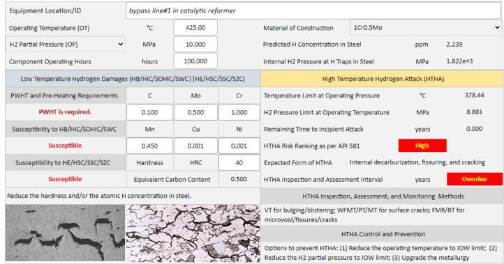
Figure 3 H2Compass Predicts susceptibility of 1Cr0.5Mo to high temperature hydrogen attack (HTHA).
