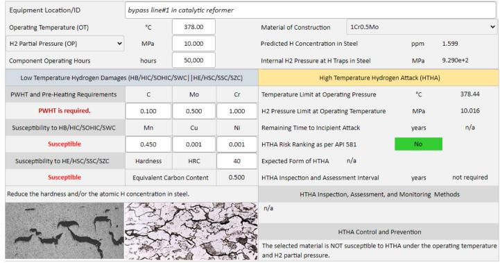
Figure 4 Reducing the operating temperature to the predicted integrity operating windows (IoWs) for high temperature high pressure hydrogen services.
