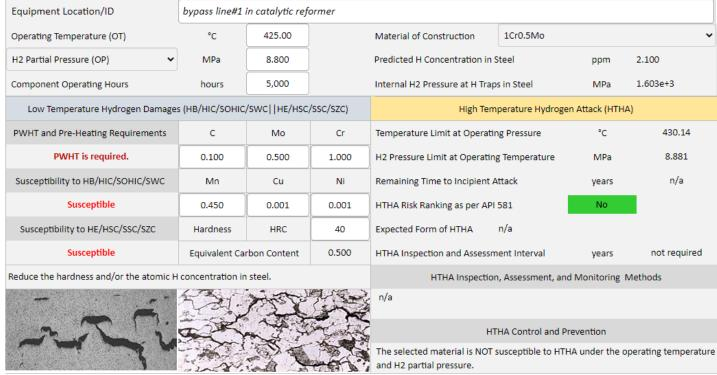
Figure 5 Reducing the operating pressure to the predicted integrity operating windows (IoWs) for high temperature high pressure hydrogen services.
