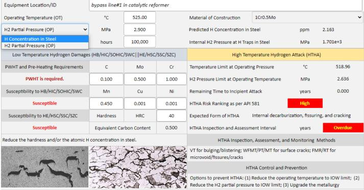
Figure 8 Hydrogen concentration in steel is used as input to assess the risk of low temperature hydrogen damages.
