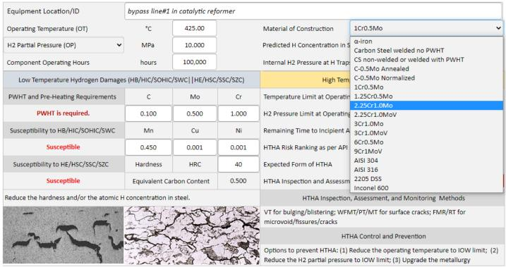
Figure 6 H2Compass for evaluation and verification of alloy selection for high temperature high pressure hydrogen services.
