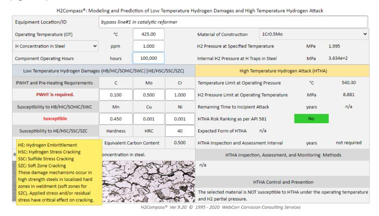
Figure 10 H2Compass predicts the concentration of dissolved hydrogen in steels and alloys and the susceptibility to low temperature hydrogen damages.
